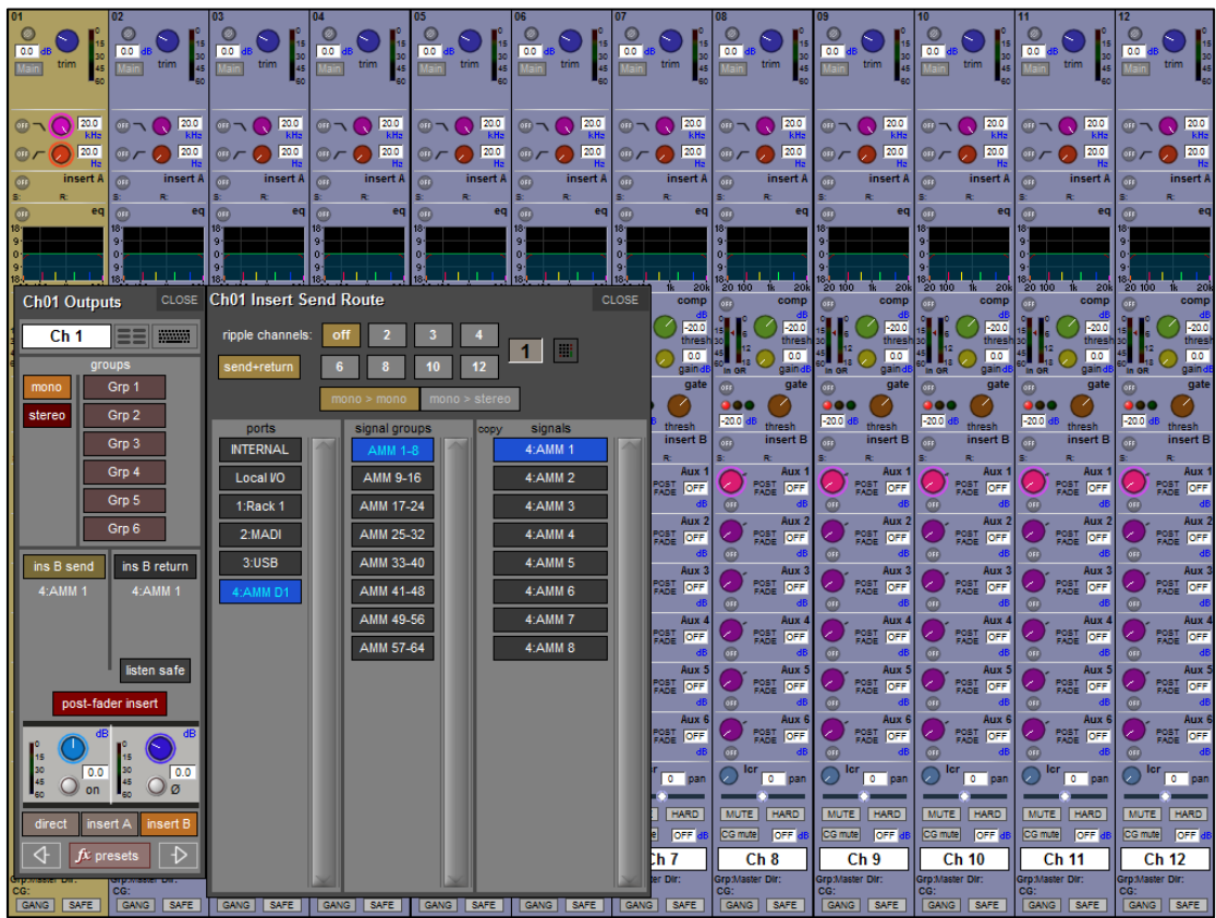
Figure 4: Routing Within AMM Control
