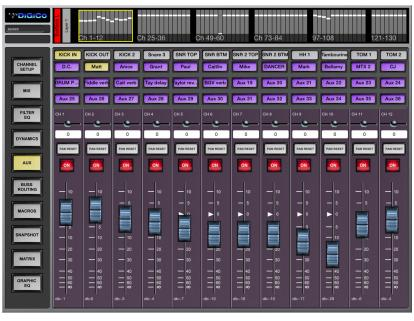
The Aux page will display auxiliary send levels, on/off, auxiliary pans.
