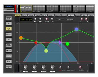
The Filter/EQ page will display 4 band Post Insert EQ, HPF/LPF, EQ On/Off, Curve setting, Bell/Precision setting and Dynamic EQ parameters
