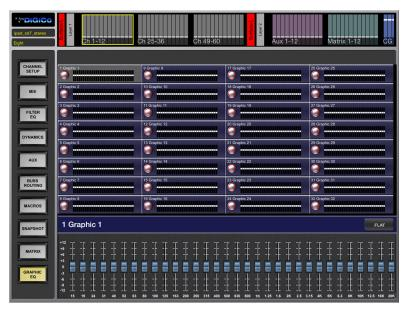
The Graphic EQ page will display 32 faders and on/off button for each unit plus a flatten all bands button for the selected unit.
