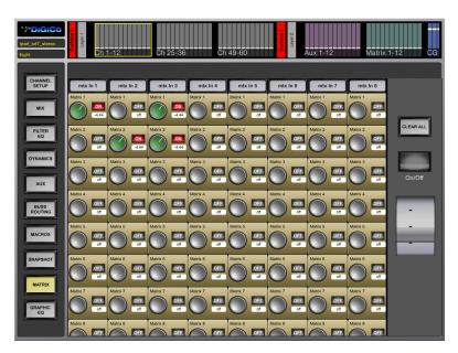
The Matrix page will display Matrix sends, on/off and matrix input labels.
