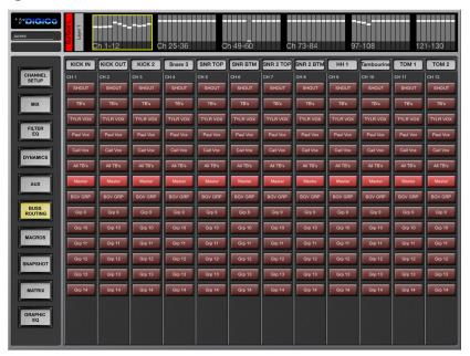
The Buss Routing page allows the assignment of input or group channels to busses.
