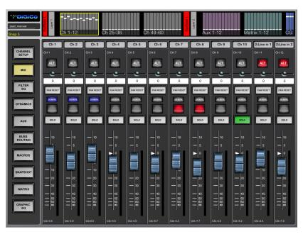
The Mix page will display Main/Alt input switch, pan, mute, solo, fader level and meters.
