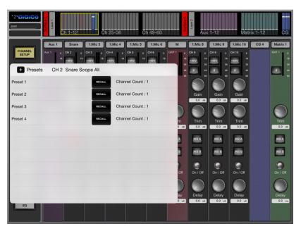
The DiGiCo SD App also provides access to the connected console's Presets library. Presets can be displayed, recalled and created.
