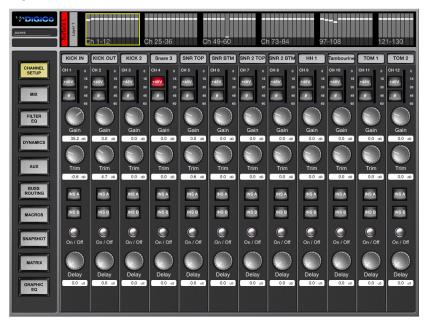
The Channel Setup page will display +48V, polarity, analogue gain, digital trim, channel delay, insert points on/off and meters.
