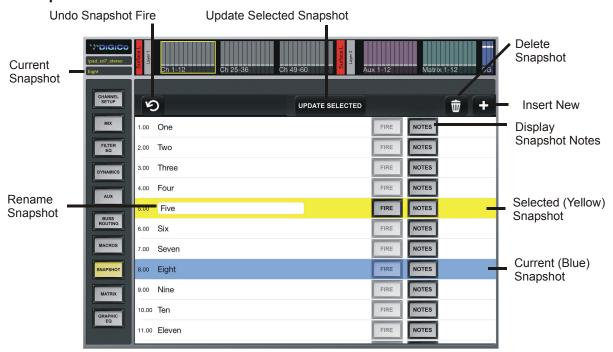
The Snapshot page allows access to the following functions - insert new, recall, undo, update, rename, delete, display notes.
