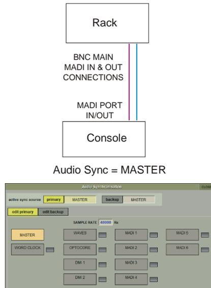
Connect Console MADI BNC IN socket to Rack BNC OUT MAIN socket.
