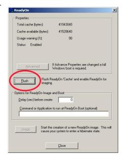
Click on the Flush Button, as indicated above. The following Progress Bar will appear. Once the Flush is complete, close ReadyOn.
