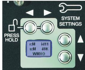
The LCD Menu System on the SD Rack MADIPod is normally in a locked state and cannot be accessed. The main display will be visible and if the rack is not connected to an SD console the background colour will be light blue.
