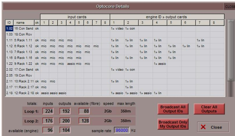
The Optocore Details Panel (shown above) shows the number of inputs and outputs mapped on each loop, the number of fibre channels available on each loop and the number of engine inputs and engine outputs remaining.
