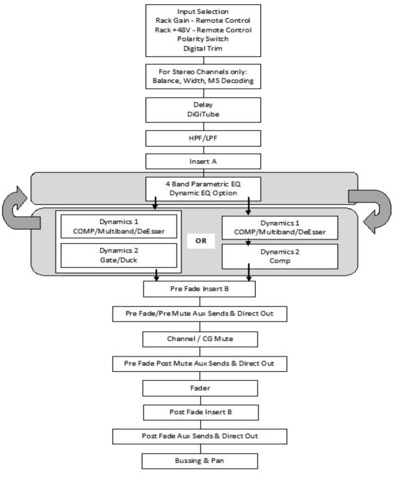
NOTE: Hard Mute stops all audio passing after the Digital Trim stage of the input module
