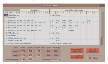
The Optocore Details Panel (shown above) shows the number of inputs and outputs mapped on each loop, the number of fibre channels available on each loop and the number of engine inputs and engine outputs remaining.
