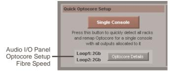
Connect all consoles and racks ensuring all Fibre connections are A to B.
