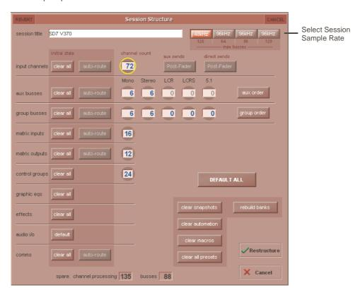
Next, go to Setup/Audio Sync and set sync to Optocore. Please note that all consoles on the network must be running at the same sample rate.
