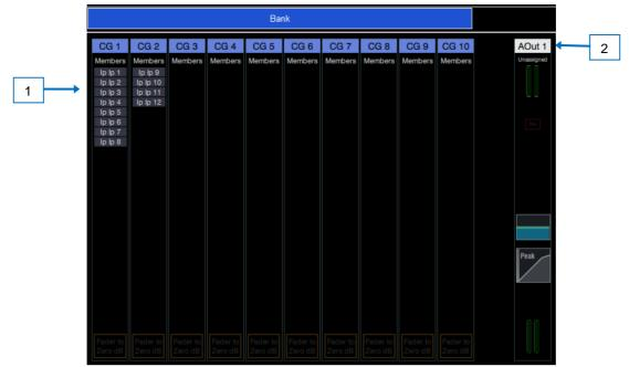
**CGs** – Displays name, members (assigned channels) and whether the 'Fader to Zero dB' option is enabled. Use the **Bussing** screen to assign channels.
