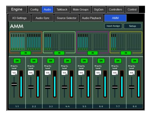
The AMM uses a 'constant gain sharing' algorithm to dynamically adjust the gain for each mic proportional to its input level. Louder signals will receive more gain in the mix.
