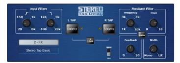
**Stereo Tap Delay -** Provides a clean digital delay with a maximum delay time of 2.7 seconds. One of the key features of the stereo tap delay is the ability to synchronise the delay times to note intervals based on the effects beats per minute value. The delay has two modes of operation:
