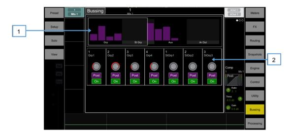
**Matrix sends** – Displays routing and assignments of Groups, Aux and Area Out mixes to the selected Matrix.
