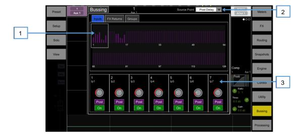
**Aux and FX sends** – Displays routing and assignments of Input channels, FX Returns and Groups to the selected Mix.
