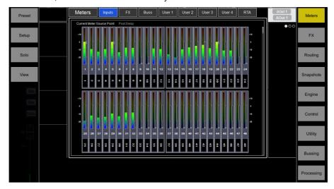
**Meters tabs** – Channel name is shown below each meter. A gain reduction meter and gate active indicator are also displayed, these show activity in red when switched In, and in grey when switched out.
