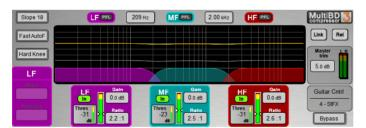
**Multiband Compressor** - Two multiband compressor types provide independent compression control over different frequency bands. This is an advanced mixing tool for mastering and live sound control. It gives more precise control over the dynamics and less pumping effect than the more common single band compressor.
