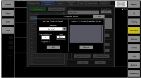
Set the **Snapshot Number** to select the Snapshot you wish to recall. Its name is displayed below the box. Set the **Delay** time for the snapshot recall. This is the time the system waits before recalling the Snapshot after you have recalled the host Snapshot. Time can be set from 0 sec (instant) to 4 minutes. Click **Add** to add the Snapshot to the list on the right.
