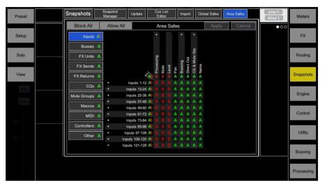
Use the tabs on the left to view the different parameter groups. Scroll to zoom in and out of the matrix view. Drag up/down or left/right to navigate through the matrix. Click an item to toggle. "Allowed" items will be recalled, "Safed" items will not.
