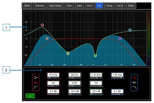
Graph – Click and drag the 4 band dots to adjust their centre frequencies. Click and drag the HPF / LPF dots to adjust their cut-off frequencies. The overall frequency response curve is highlighted when the EQ is switched in and dim when switched out.
