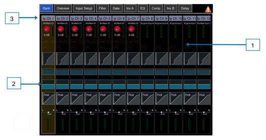
**Input channels** – Displays name, source type, input meter, gain, +48V and polarity, gate graph, filters, EQ graph, compressor graph, pan and channel meter.
