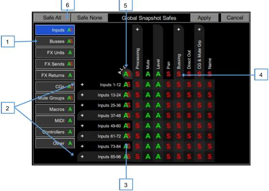
Scroll to zoom in and out of the matrix view. Drag up/down or left/right to navigate through the table. Click an item to toggle its state.
