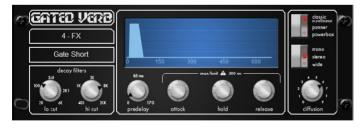
**Gated Verb** - An accurate emulation of the classic 80's Gated Reverb plus two other variants called 'Panned' and 'Powerbox'. The user interface gives instant access to Lo-cut Hi-cut decay spectrum filters and the gate envelope controls - predelay, attack, hold and release.
