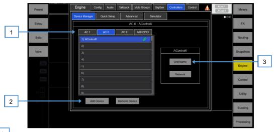
Select the device tab using the tabs on top and select one of the 16 locations in the list. The list shows the unit name of assigned devices.
