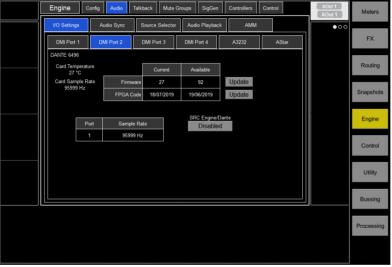
DMI Dante 64@96 allows 64 channels at 96kHz. It behaves and is controlled in the same way as the original DMI Dante, with the addition of SRC. SRC is supported down to a Dante network running at 48Khz and is enabled by clicking the "Disabled" button beneath "SRC Engine/Dante".
