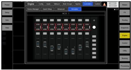
Click a button on the screen to control the assigned function. Click and drag a fader / rotary control to control the assigned parameter.
