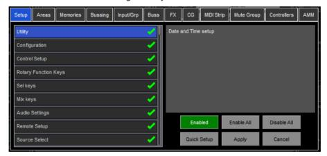
**User permissions** – Each User can have their own set of Permissions applied. Use the tabs across the top of the window to view and set different groups of permissions. Select an item in the list and toggle the **Enabled/Disabled** button as required. The window on the right provides a description of the functions included in the currently selected item. Use the **Enable All / Disable All** buttons to quickly toggle all items in the currently open tab. Click **Apply** to accept the changes.
