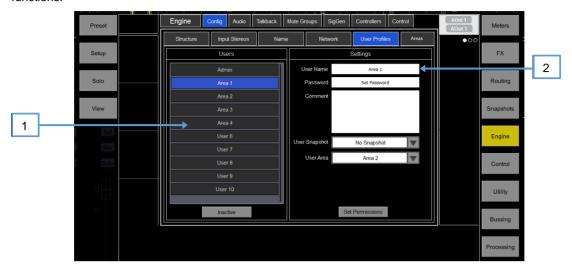
Users – The Admin user has access to all functions and can set permissions and allocate passwords if required for the other users. The password, if one is set, is required when the User logs in or changes User. Icons in the list indicate if a password is set and if the User is active.
