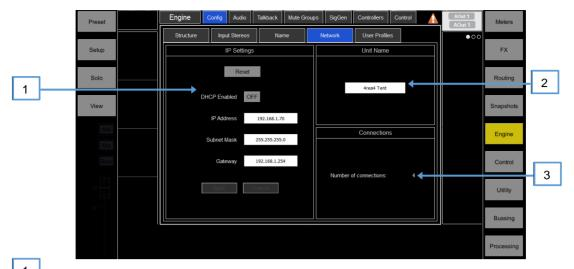
IP Settings – To set a static IP Address, click the IP Address box and type in the address. Make sure the Subnet Mask and Gateway are valid, and all devices on the network including Wi-Fi routers, access points or laptops have unique but compatible addresses.
