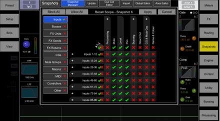
Use the tabs on the left to view the different parameter groups. scroll to zoom in and out of the matrix view. Drag up/down or left/right to navigate through the matrix. Click an item to toggle. Allowed items will be recalled, Blocked items will not.
