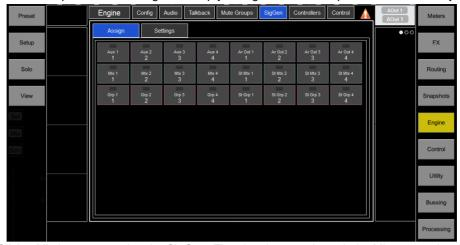
**Assign** – Click a Mix button to assign the SigGen. The signal routes through the Mix processing, therefore will be affected by the Mix EQ and compressor.
