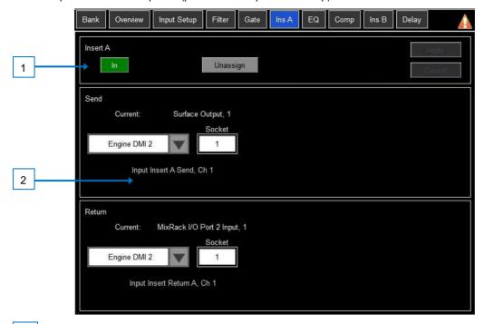
Insert Settings – Click In to switch the inserted device in circuit. Click Unassign to clear the current Insert assignment.
