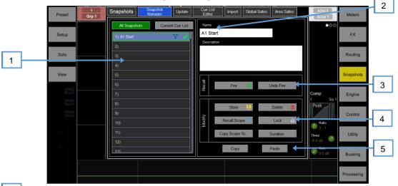
Snapshot list – Choose to display the list of all 800 snapshots or the Current Cue List. The snapshot highlighted in blue is the currently selected snapshot and is displayed in the bottom left corner of the snapshot panel. The snapshot highlighted in green is the next snapshot and is displayed in bottom right corner of the snapshot panel.
