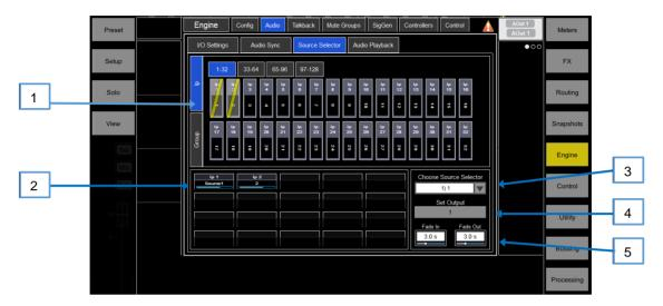
Sources: Inputs / Groups – Use the vertical tabs to switch between inputs and groups. Drag and drop inputs and/or groups into the lower pane to add them to a Source Select group.
