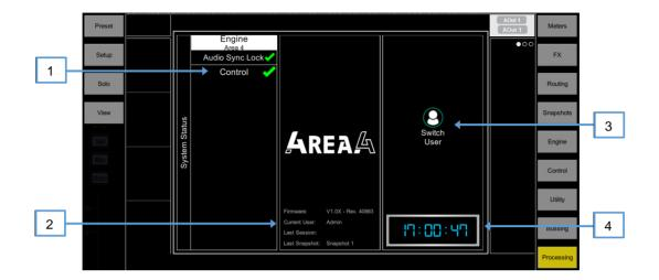
System Status – Displays a list of system components. A green tick indicates the component is running correctly. A red cross indicates that an error is detected. A blue icon appears when a non-critical event is logged. Click the component to display further information.
