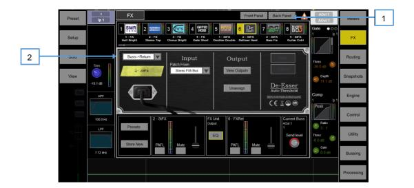
Back Panel – Use this view to edit the routing for the selected FX. Use the drop-down box to choose between Unassigned, Insert or Buss->Return.
