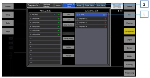
Current Cue List – Drag and drop snapshots here to create a Cue List. Snapshots can be placed in any order and repeated any number of times in the list. To remove a snapshot from the Cue List, click the trash can icon to the right of the snapshot name.
