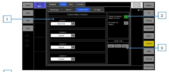
Custom Rotary Functions— Use the drop-down menus to select the required Function for each Custom strip rotary control. Available functions are Unused, Direct Out, Send Level (Aux or FX sends), HPF Frequency, Compressor Threshold, and Channel Level. Click **Apply** to confirm the change.
