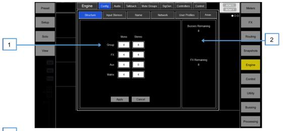
Bus configuration – Click and drag a box to set the number of mono / stereo Groups, FX sends, Aux sends and Matrix outputs. You can choose any combination but note that mono busses can only be added / removed in pairs.
