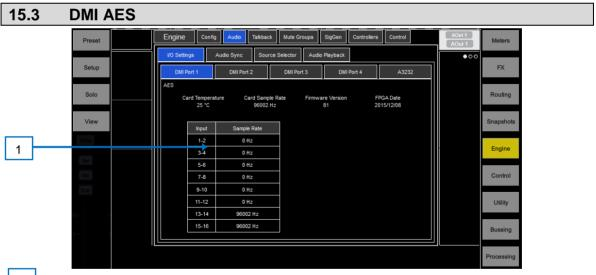
Input SRC Display – Enable the SRC Bypass option in Routing view by clicking on the relevant socket to disable input sample rate conversion on a socket pair basis.
