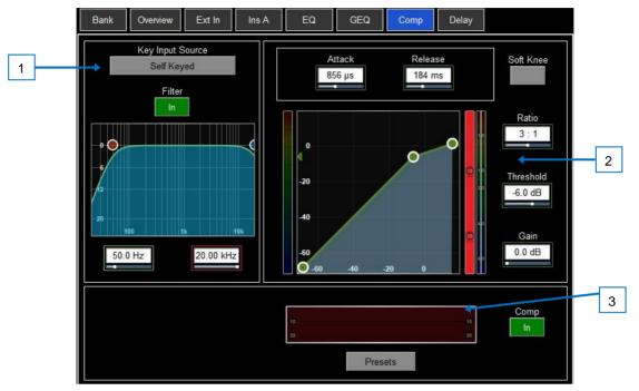
Side Chain – Click the **Key Input Source** box to open a window for selecting the Key (trigger) input to the Compressor. An adjustable HPF and LPF filter can be switched in to limit the frequency range of the Key signal.
