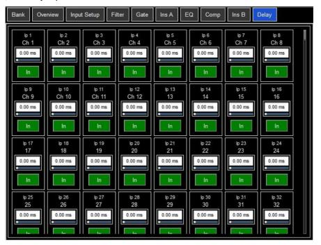
• Click Setup and then click anywhere in the Delay page to access the unit and temperature preferences for the Delay. The default unit is ms but can be changed to metres, feet, or samples. This can be changed globally for the Input channels and for the Mix channels. Enter the ambient temperature if using distances so that 4REA4 can compensate for the effect on delay.
