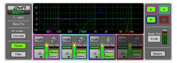
**Dynamic EQ -** DynEQ4 is a model of the industry standard stereo 4-band Dynamic Equaliser. It is an advanced processing tool providing four bands of equalisation that respond to the dynamics of the signal.
