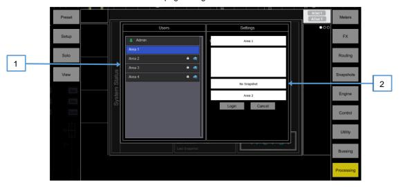
Users list - Shows available Users. These can be configured and enabled in the Engine / Config / User Profiles screen. The Admin User is always displayed. Icons indicate if the User has a password or User Snapshot set. Click a User to select then click Login to change User.
