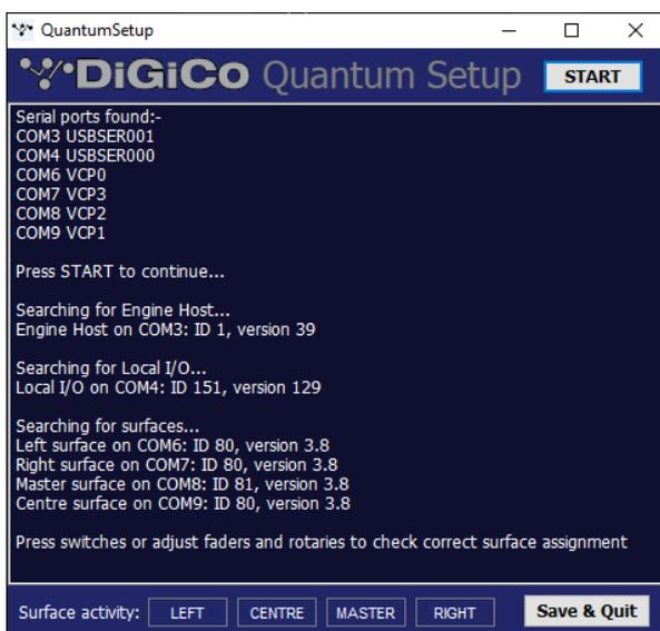
8. Adjusting any control on each worksurface will highlight the appropriate Worksurface activity button as shown.
