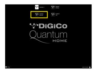
In Quantum Upgrade, for each device, you will see the current running version in the "running" column, with the new version in the "available" column. The available version is based on the corresponding file in D:\QUANTUM8 directory.
