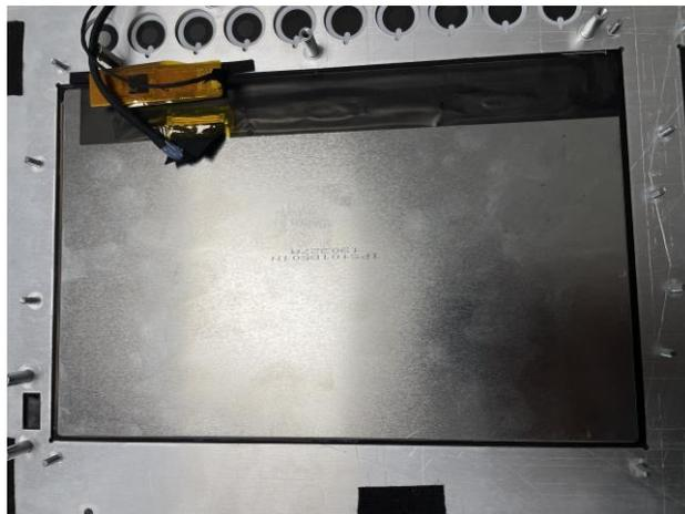
Step 3 – Re install the metal bracket to the panel and secure with the M3 nuts.
