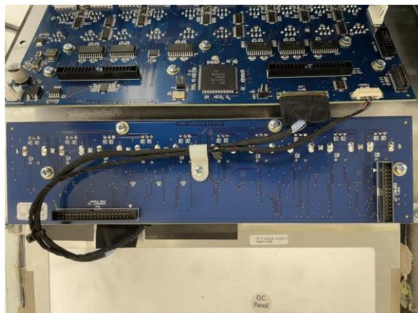
Step 5 – Reconnect the Touchscreen driver cable and touch cable to the fader driver card.
