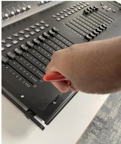
Step 3 – Slowly lift the lower section first and disconnect the power and grey ribbon cable from the fader driver PCB which frees up the front panel to be removed from the console chassis.
