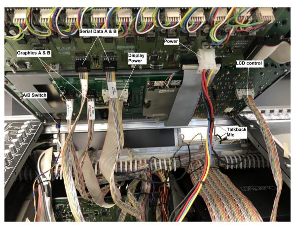
Locate the local I/O backplane board. Disconnect cable connections as shown below. Note that it is recommended to remove the video clamp PCB from the video switcher board to allow the PSU connectors on the local I/O backplane to be removed more easily.
