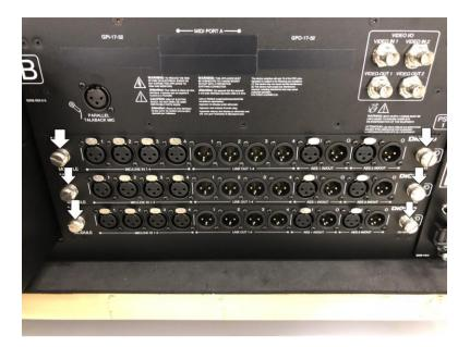
Remove 6 x 2mm kex stainless panel fixing screws from the master upper panel (Use the 2mm hex driver). Lift the upper surface from the bottom edge (nearest faders). Disconnect cable connections as shown below and remove the surface.
