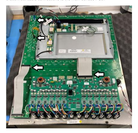
Unscrew and remove the main surface board.
