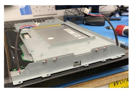
Unscrew the rear bracket from the display to release the display from the bracket.
