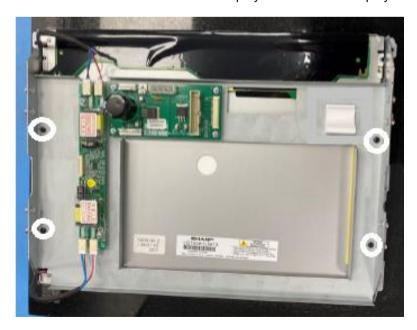
Replace display and perform steps in reverse to reassemble.
