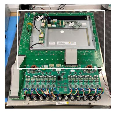
Disconnect graphics cable between the display and graphics interface board.
