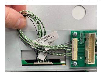
Disconnect Display inverter from the display backlights.
