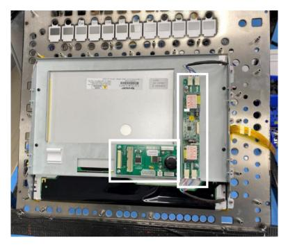
Remove the M3 SL nuts that are securing the side brackets to the panel.
