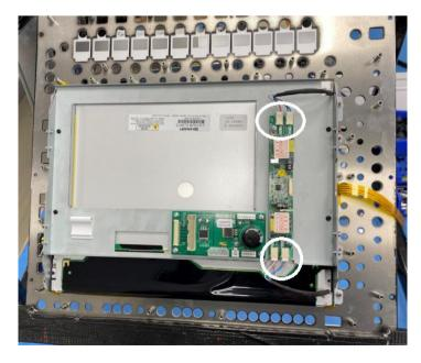
If either the Display inverter board or graphics interface board PA16098 are required to be replaced they can be unscrewed and removed from the bracket
