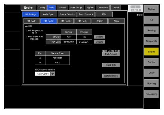
With an SD console connected via Optocore to the 4REA4, the Input Channel Count and Output Channel Count should be set to the number of channels that need to be controlled. The SD console can also be connected via MADI to the 4REA4 with the MADI Mode Selection set to "SD Console."
