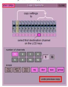
Figure 7 - Copy Channel Display
