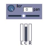
Note: the pan of the Assigned channel can be controlled using the worksurface joystick (SD5,7,8,10). The pan control can also be assigned to one of the encoder rows. LR/LCR Blend is adjusted using the 2nd function button.
