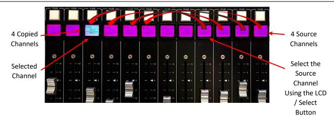
Figure 6 - LCD Copy Functions
