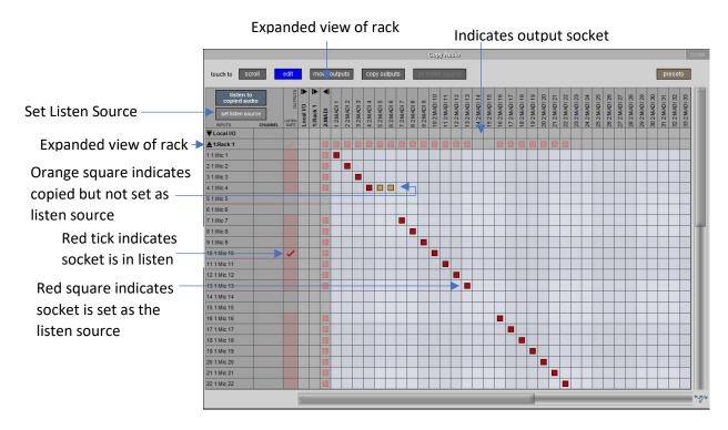
Open the Master Screen / Setup / Copy Audio panel and you will see the collapsed matrix with input ports listed down the left side and output ports across the top.
