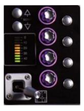
The auxes controlled by these encoders and buttons can be selected using the scroll buttons to the left of the top encoder and is indicated by purple ring on the on-screen aux sends.
