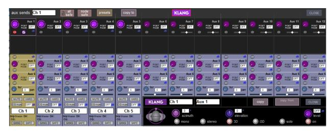
KLANG Nodes can be activated on aux send to allow control of the channel's KLANG parameters. A KLANG button is displayed in expanded aux panel and the Aux Nodes panel after KLANG is enabled in the External Control panel (See Chapter 2 - 2.12.14).
