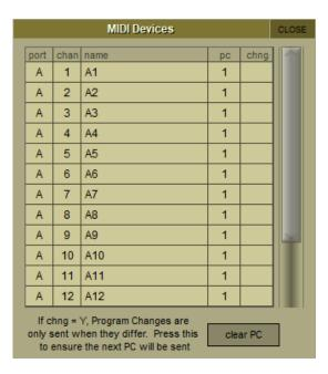
The SD Console's built in MIDI port is referred to as Port A in the **Port** column. Set the receiving MIDI **chan**nel and **name** for each of your receiving devices and set 1 or 0 in the **PC** column according to whether the device uses 0-127 (0) or 1-128 (1) for its data values. If you don't know this piece of information, then leave the setting as 1.
