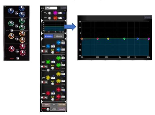
In both the EQ/filters display and on the worksurface, each band has a ±18dB gain controller on the left, a frequency controller (ranging from 20Hz to 20kHz) top right and a Q control bottom right. Each rotary has its value displayed to its right.
