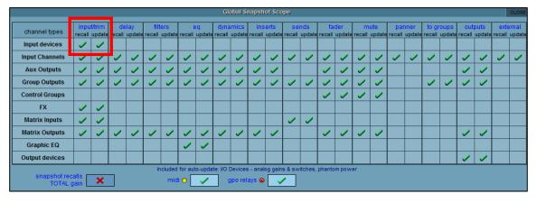
Figure 8: Global Scope > Input Devices
