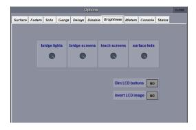
The SD5 and SD7 console's LCD buttons are not controlled by the **surface LEDs** pot but by the **Dim LCD buttons** and **Invert LCD Image** options towards the bottom of the screen.
