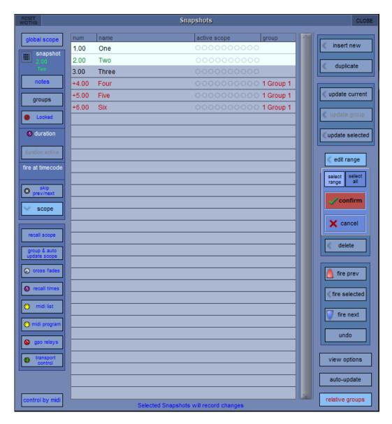
With the **Edit Range** button active, pressing the Snapshot buttons does not fire the snapshots; it only selects them for editing. The selection may be changed by pressing and releasing snapshot buttons at any time during the operation of the Edit command, so a variety of controllers or routes may be changed in a variety of snapshots before completing the operation by pressing the **Confirm** button. The Snapshots window may even
