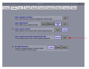
To avoid delaying fader input when recalling Snapshots/Cues select Fast option.
