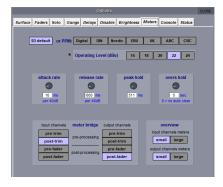
The four pots across the middle of the panel affect the attack and release reaction time (attack rate and release rate), the peak hold time and the overs hold time. The current setting for each is displayed in either milliseconds or seconds, below each pot. Touching each pot assigns it to the Touch-Turn encoder. The row of
