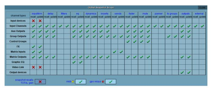
Horizontal rows show the different sections of the console and the vertical rows show the Recall and Auto Update status for each of the different types of control. A red X indicates not included and a green tick indicates included. These settings can be changed individually by touching the X or tick symbols or by touching the name of a row or column to change all of its contents.
