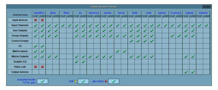
Horizontal rows show the different sections of the console and the vertical rows show the Recall and Auto Update status for each of the different types of control. A red X indicates not included and a green tick indicates included. These settings can be changed individually by touching the X or tick symbols or by touching the name of a row or column to change all of its contents.
