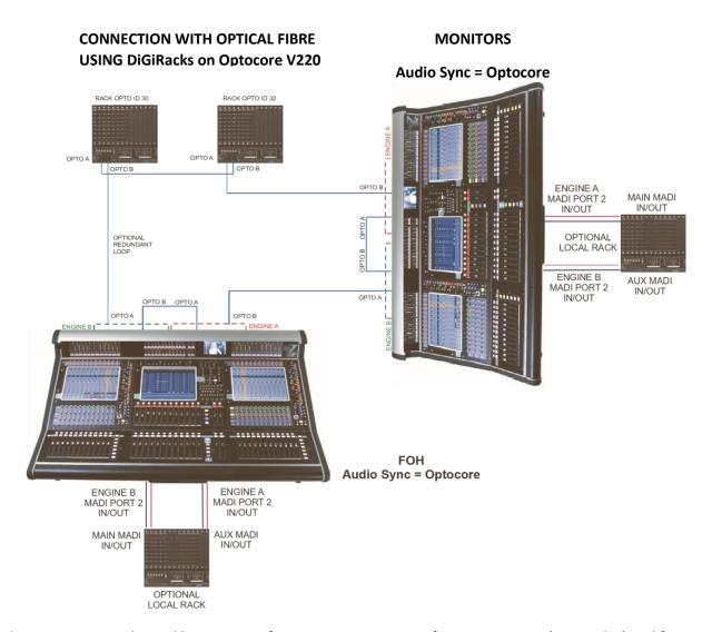
In this setup, you are limited by Optocore firmware Version 220 to four SD7 engines (2 consoles) and four Optocore connected racks. The system can only run at a sample rate of 48KHz.
