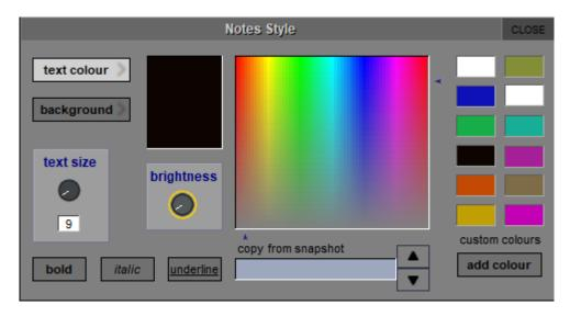
The text can be formatted using the **text size** controller and **bold**, **italic** and **underline** buttons in the left side of the panel. To change the colour of the text or background, select either the **text colour** or **background** button in the left side of the panel, touch inside the colour palette in the centre of the panel, and adjust the brightness using the **brightness** controller. The selected colour is displayed above the **brightness** controller.
