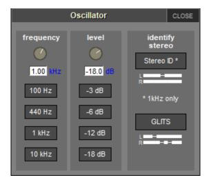
The frequency of the oscillator is controlled by the left-hand **frequency** on-screen rotary, and its audio level is controlled by the right-hand **level** rotary. The buttons below each rotary, can be used to set the oscillator to standard frequencies (**100Hz**, **440Hz**, **1kHz**, **10kHz**) and levels (**-3dB**, **-6dB**, **-12dB**, **-18dB**). The current value of each parameter is displayed below its respective rotary.
