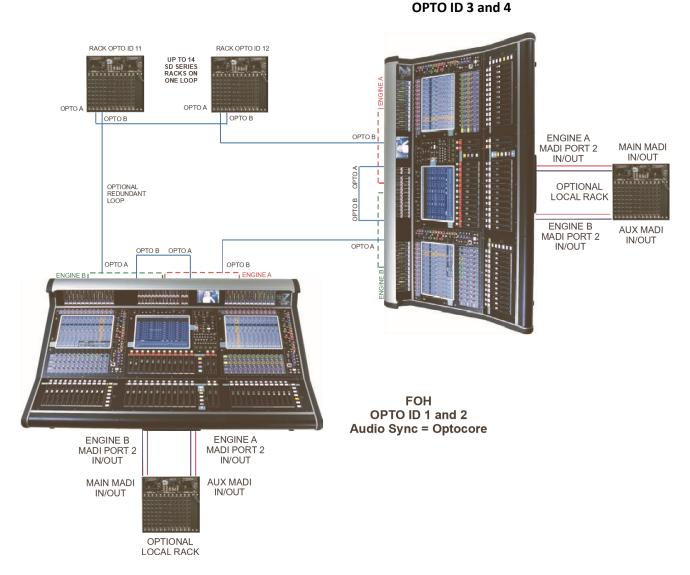
It is possible for up to 5 DiGiCo consoles to share the inputs from remote stage SD Racks using optical fibre cables. It is also possible for the output cards in the SD Racks to be allocated to the consoles on a card by card basis.
