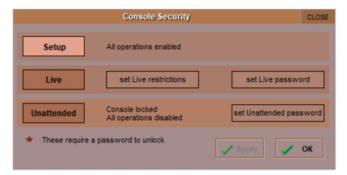
User passwords can be defined for the Live and Unattended modes. To set a password, press the **Set Password** button. Enter the old password then the new one twice and press **OK**. By default, the passwords are blank.
