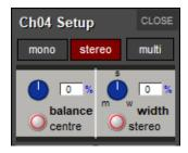
Stereo channels also have an m-s button, located above the input routing button, which switches in a decode function for replaying M-S signals as a normal stereo pair. There are three further buttons in this panel: L<>R swaps the channel's left and right outputs, L>L+R sends the left signal to both left and right busses, and R>L+R sends the right signal to both left and right busses.
