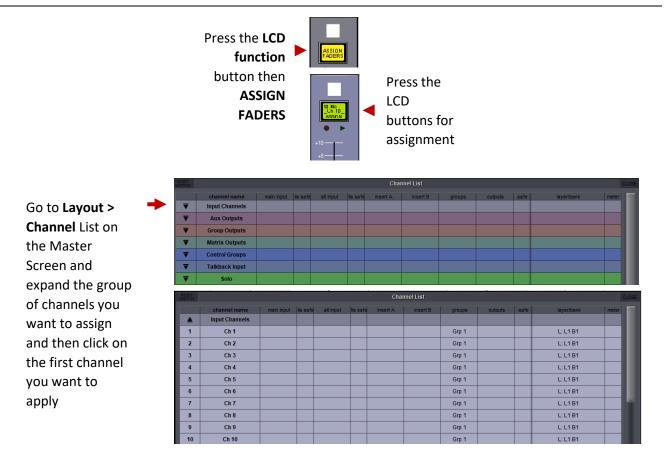
To select the channels you wish to assign to those channel strips, open up the **Channel List** display, accessed by going to the master screen and touching **Layout** > **Channel List**. There you will find a list of all input, output and control channels that are present in the session structure, grouped by channel type. Open up the channel list for the channel type of the first channel to be assigned by touching the appropriate down arrow in the left-hand column.
