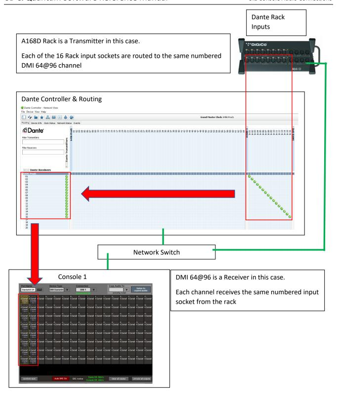
In this example, a console that routes signal to DMI card output channels 1-8 will be sending them to the same numbered Rack Output socket.
