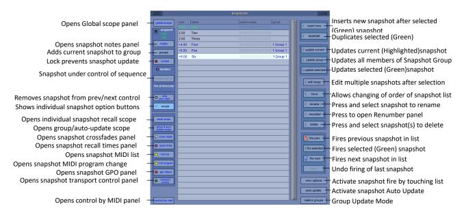
Note: The current snapshot appears in the panel as the highlighted entry in the list. The snapshot name displayed in green indicates that it is the selected snapshot on the worksurface and its name is indicated in the display. The Fire button recalls this selected snapshot and highlights it in the screen list as the current snapshot.
