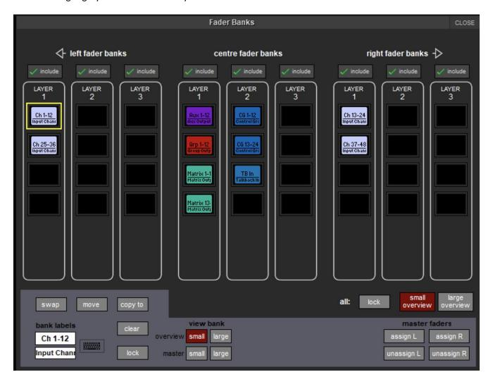
To swap the locations of two fader sets, touch one set's bank so that it is highlighted in yellow, touch **swap** (located below the left fader bank's layer 1) and touch the other set's bank.
