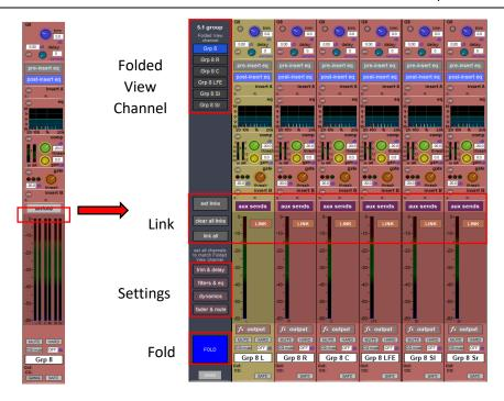
Figure 32 - Folded and Unfolded View
