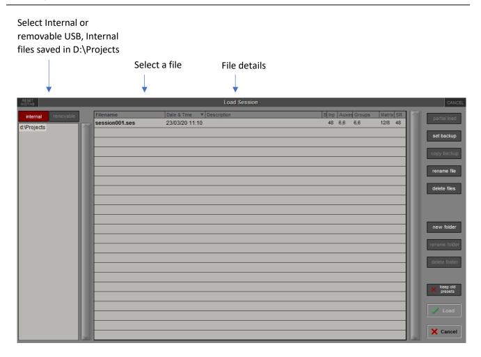
Note: that column widths can be adjusted by dragging their borders within the title row. To return all columns to their default widths, press RESET WIDTHS, in the top left-hand corner of the window.
