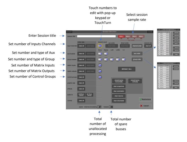
The above figure shows the SD7 Session Structure Panel. Pressing the Default All button followed by the Restructure button will automatically configure a new session where the inputs from Audio I/O Port 1 are routed to input channels and the Master Buss is routed to Local outputs 1 & 2, also to Port 1 rack outputs 1 & 2. All input channels will be routed to the Master Buss and the console headphones will be fed by the Master Buss when nothing else is soloed.
