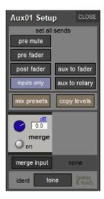
The set all sends buttons at the top of the Setup display affect the sends to that aux bus from all of the Input channels. The three buttons on the left, pre mute, pre fader and post fader, set the point in the channel from which the aux send is taken. The current send point is displayed next to the aux send level in the Input channels.
