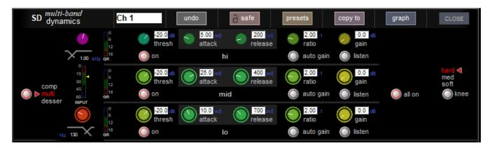
The crossover frequency between bands is controlled using the purple and red rotaries to the left of the hi and lo bands. Each crossover has a range of 20Hz to 20kHz, and the crossover frequencies are displayed below each rotary. Each band can be auditioned (destructively) by pressing the listen button below each gain rotary.
