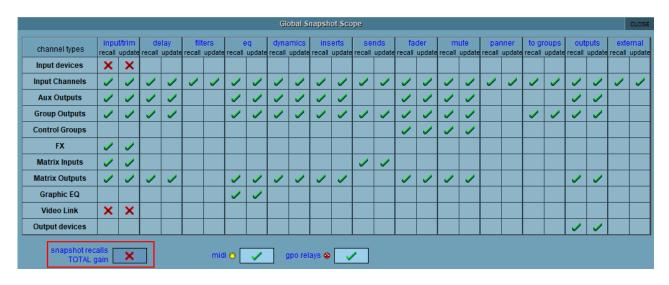
Figure 26 - Snapshot Global Scope Panel
