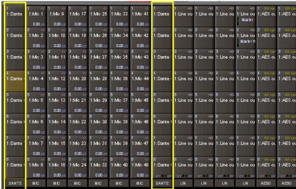
The Dante card's sockets will appear in the console's input and output routing panels and therefore routing to and from the console to the Dante card is achieved in the same way as with any other DiGiCo Input/Output card.
