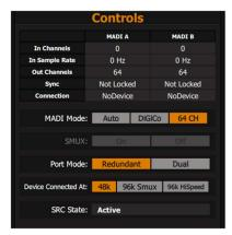
When in the Master Slot (DMI 1), the SRC controls decide the Sample rate provided to the DMI card in the Slave Slot (DMI 2).
