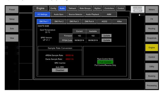
Dante IO boxes can operate at either 48K or 96K (set in Dante Controller device configuration). If the requirement is to place the IO box onto a 48K Dante Network, this is possible by setting the Dante IO box and DMI 64@96 card to 48K and activating Auto SRC to convert up to 96K from the card to the 4REA4 Engine.
