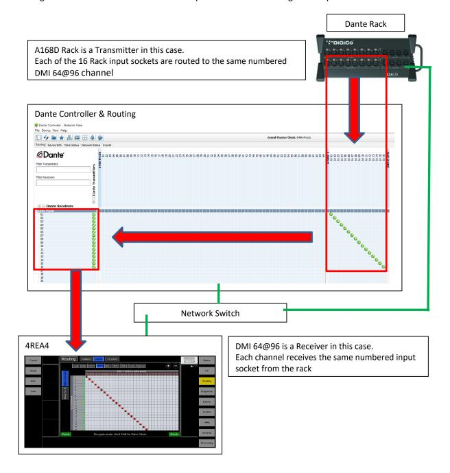
In this example, a console that routes signal to DMI card output channels 1-8 will be sending them to the same numbered Rack Output socket.
