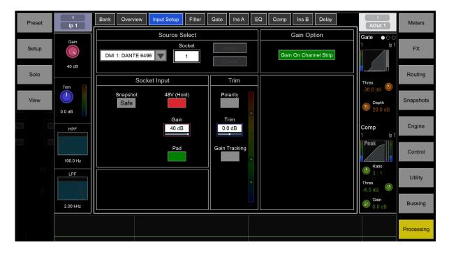
As with all other IO boxes, routing is possible both in the **Routing** matrix view and from the selected channel strip **Processing, Input Setup** view. In the case of Dante IO, the input source will be a channel number on a DMI Dante
