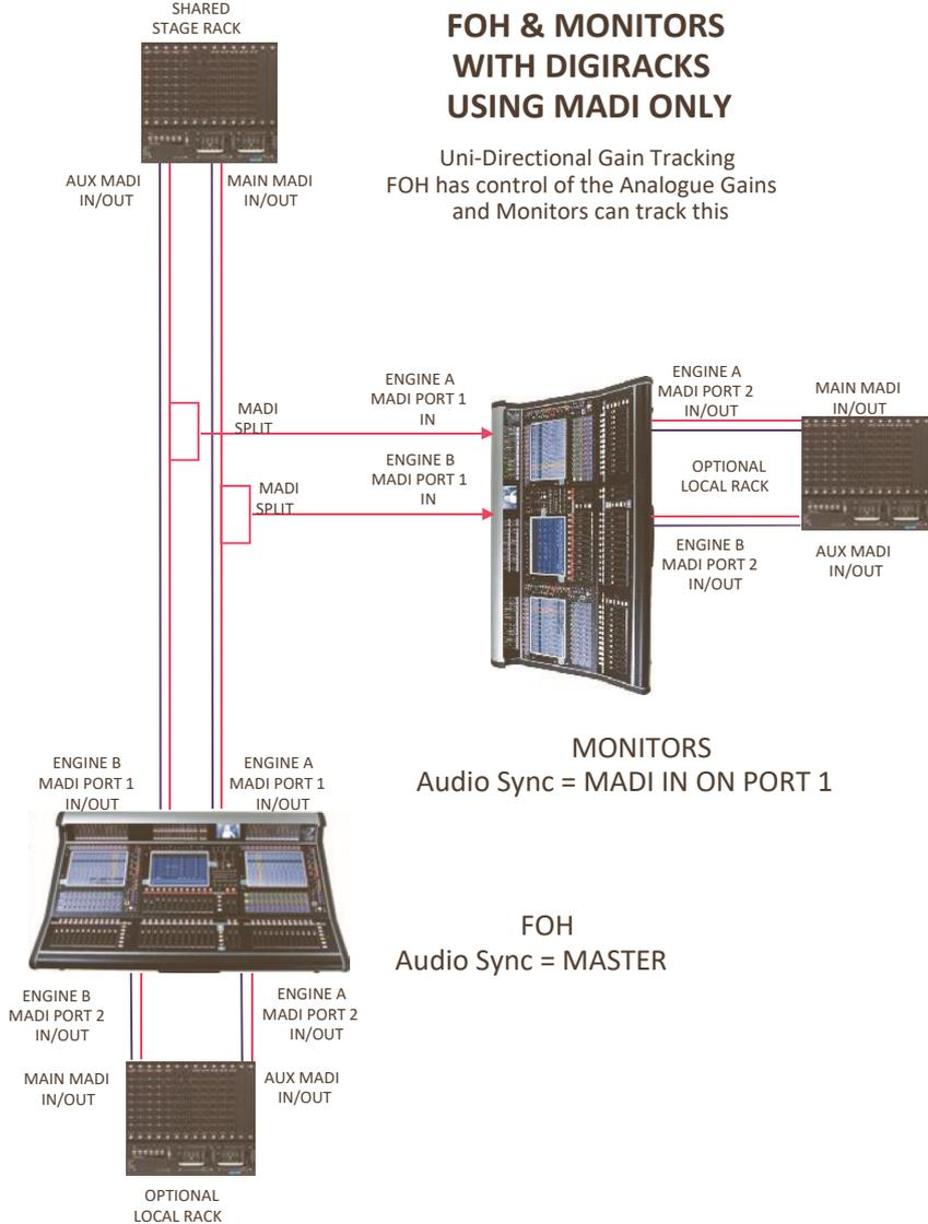
When using racks on MADI, because each SD7 has 2 engines there is a requirement to split the rack's MAIN and AUX MADI OUT signals to feed the second console's MADI IN ports.
