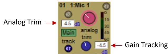
Figure 25 - Input Area of Channel Strip
