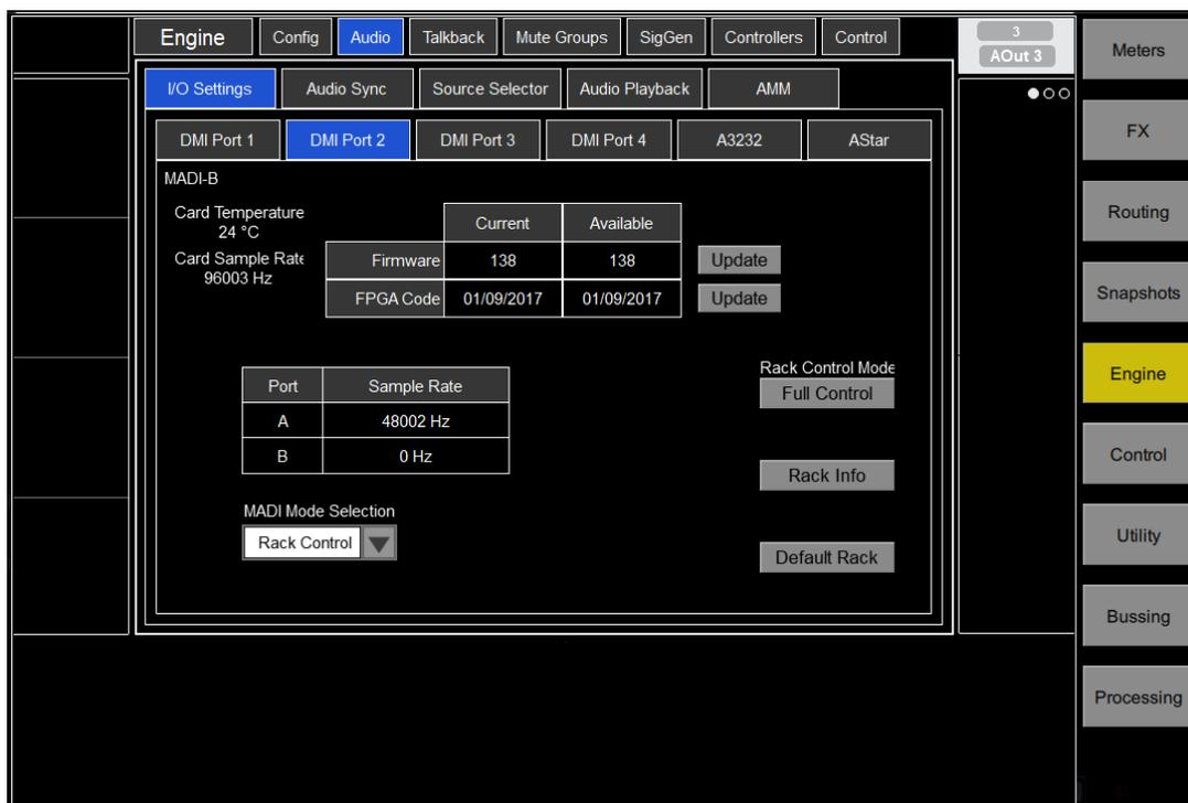
With an SD console connected via Optocore to the 4REA4, the Input Channel Count and Output Channel Count should be set to the number of channels that need to be controlled. The SD console can also be connected via MADI to the 4REA4 with the MADI Mode Selection set to “SD Console.”
