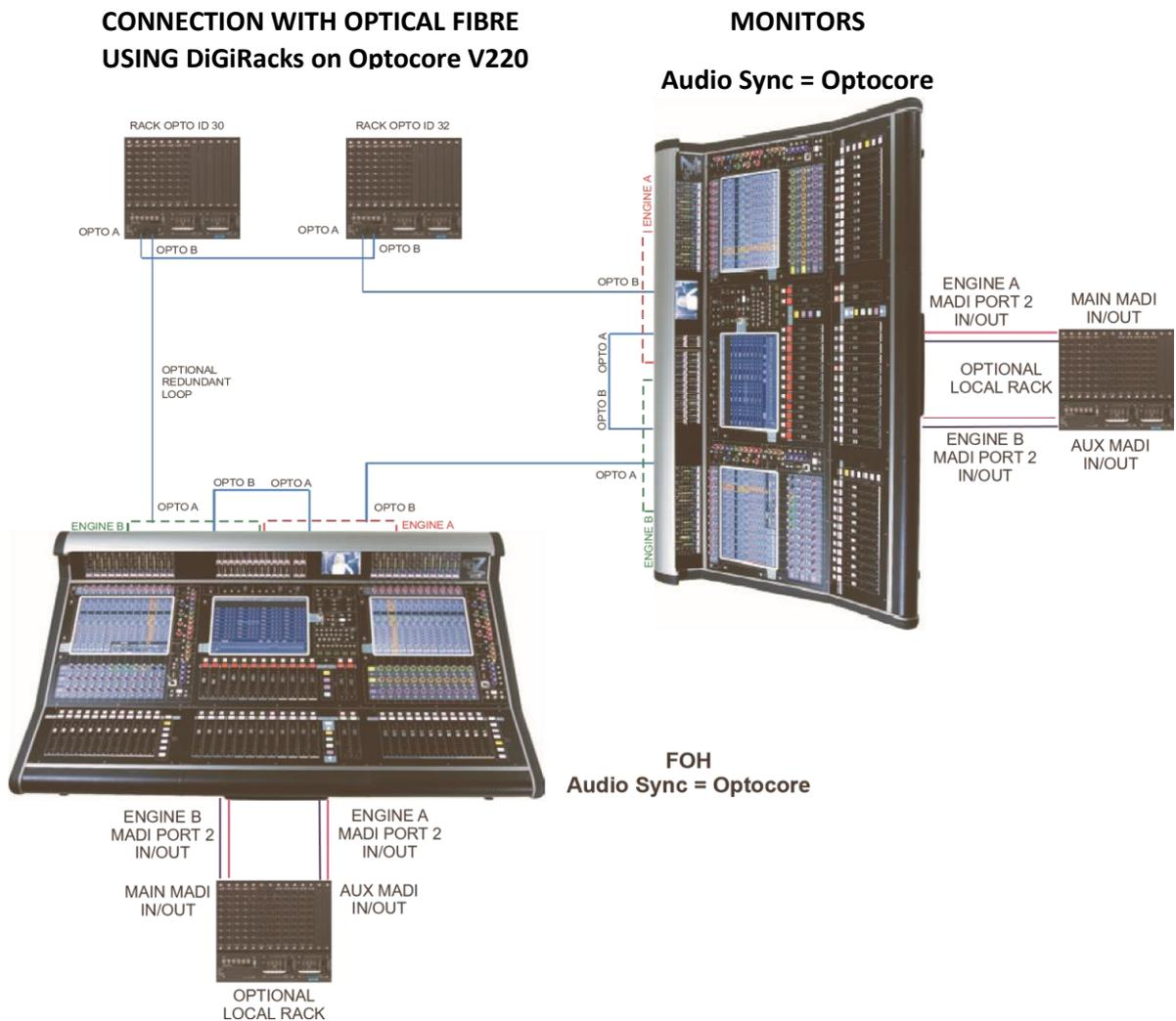
In this setup, you are limited by Optocore firmware Version 220 to four SD7 engines (2 consoles) and four Optocore connected racks. The system can only run at a sample rate of 48KHz.
