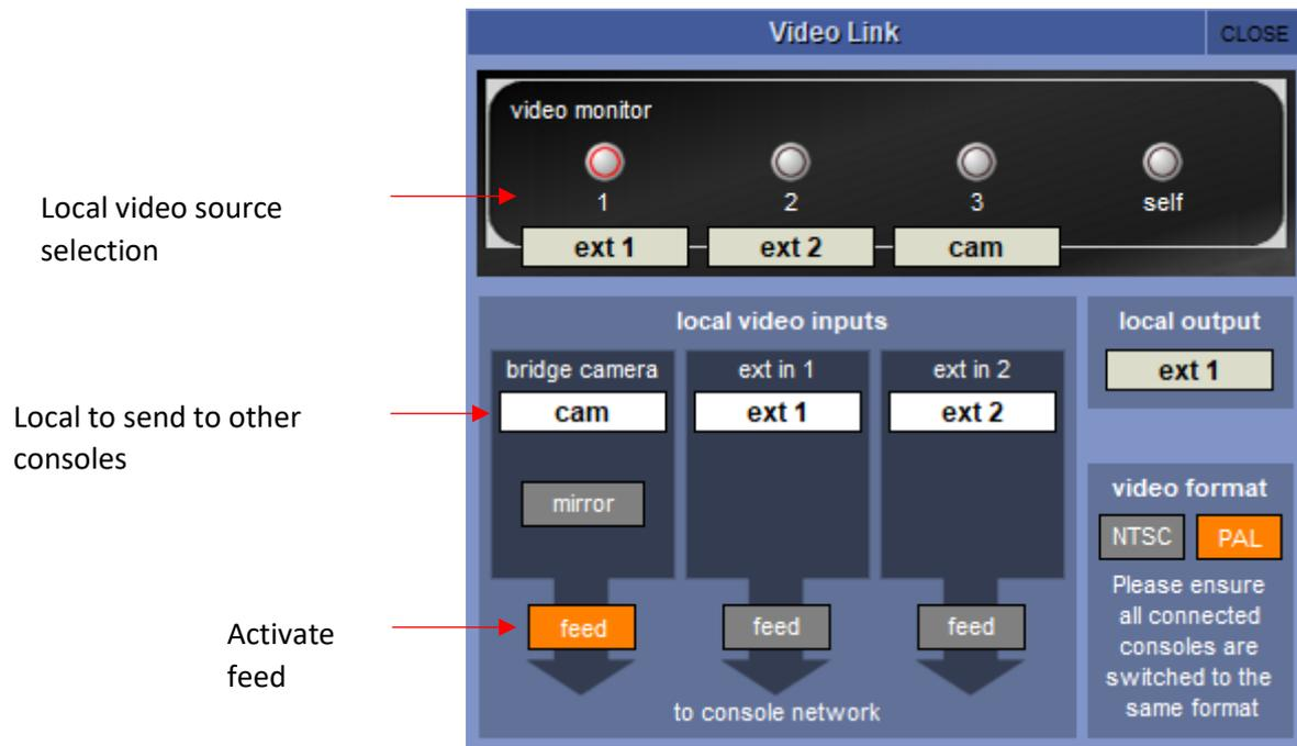
To define the source associated with each button, touch the white label box below the on-screen label and a drop-down menu will appear.
