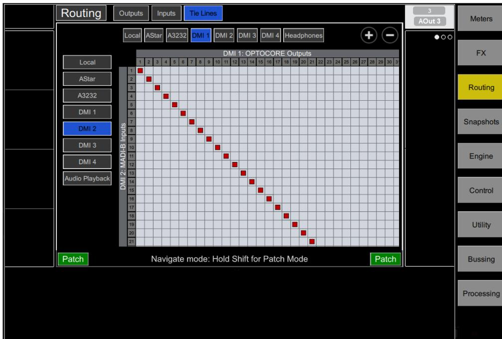
Once the 4REA4 has been set up with the correct DMi card settings and Tie Lines are in place, in the SD Console Audio IO window, a “4REA4 Port” can be added from the Add Port drop down menu and then using the Conform Port function or by using the Conform All Ports function.
