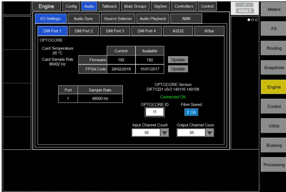
Tie Lines connecting the MADi Rack inputs to the Optocore outputs, Tie Lines can be set up in the other direction to allow output socket control. This creates a link for audio and control data. The whole IO or specific sockets can be tie lined up to a total of 64
