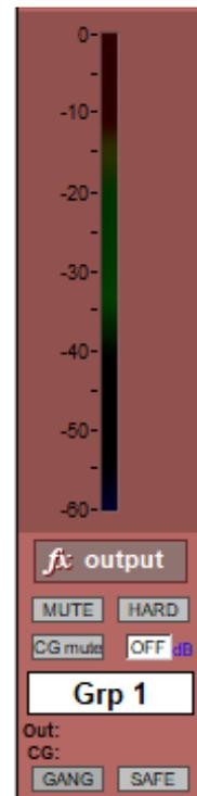
Figure 15 - Output Channel Meter
