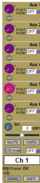
Figure 14 - Aux Send Area of Channel Strip
