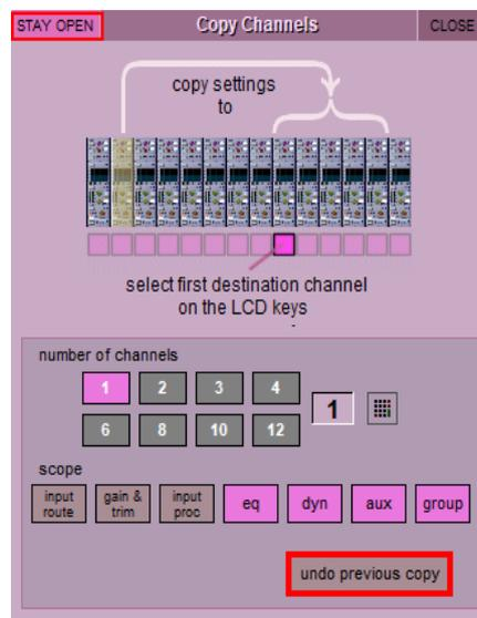
Figure 7 - Copy Channel Display
