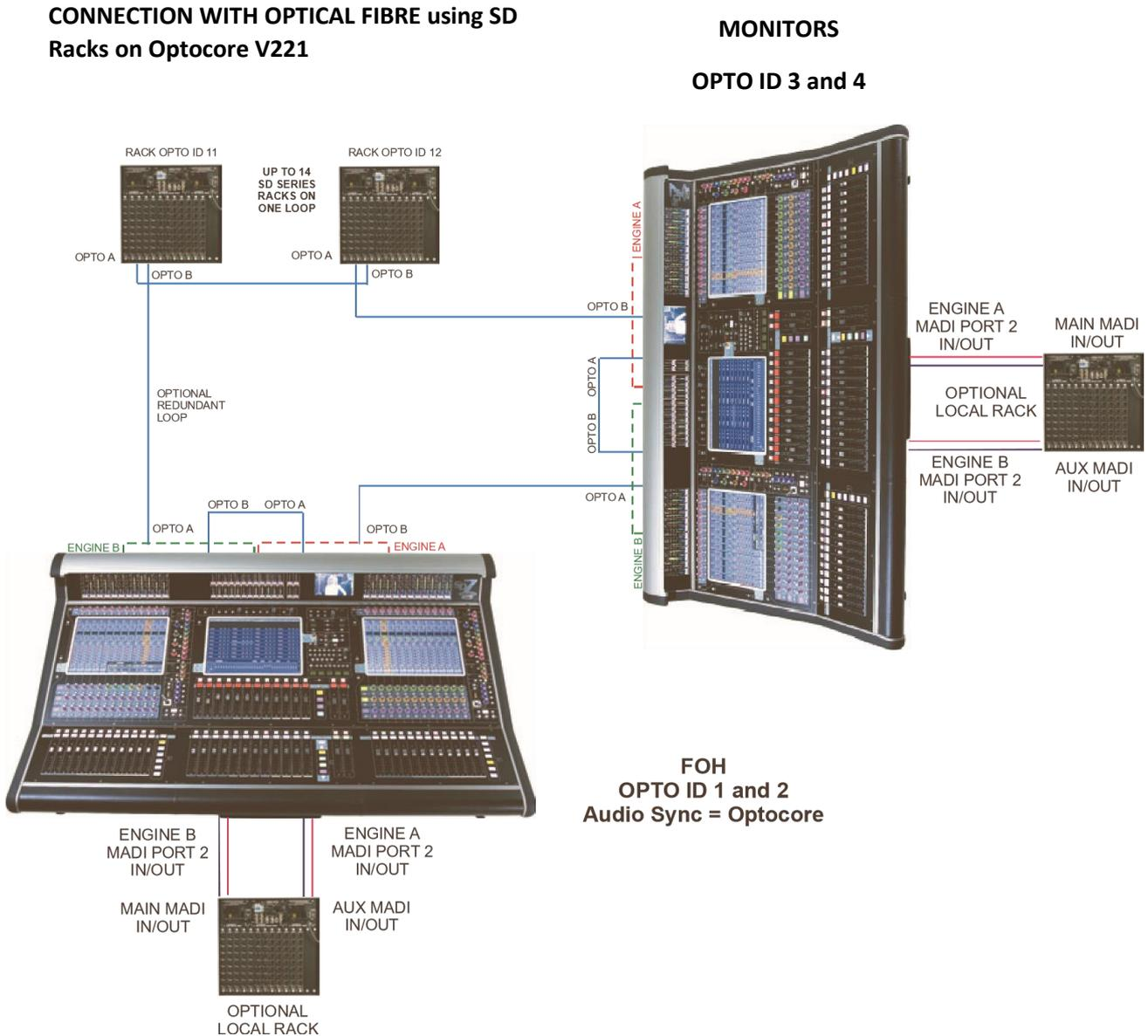
It is possible for up to 5 DiGiCo consoles to share the inputs from remote stage SD Racks using optical fibre cables. It is also possible for the output cards in the SD Racks to be allocated to the consoles on a card by card basis.
