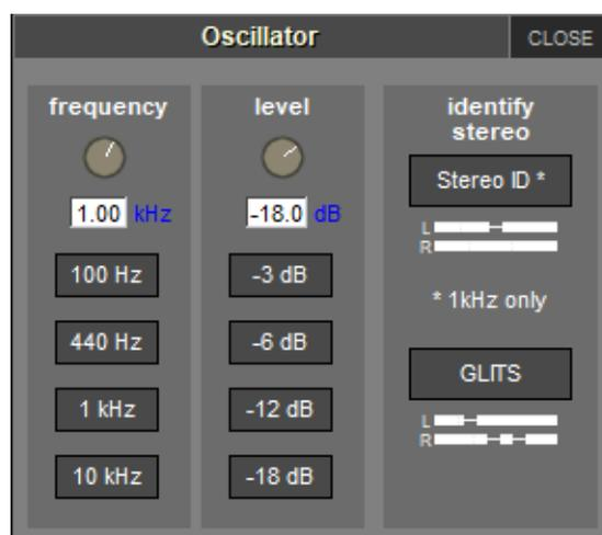
The frequency of the oscillator is controlled by the left-hand **frequency** on-screen rotary, and its audio level is controlled by the right-hand **level** rotary. The buttons below each rotary, can be used to set the oscillator to standard frequencies (**100Hz, 440Hz, 1kHz, 10kHz**) and levels (**-3dB, -6dB, -12dB, -18dB**). The current value of each parameter is displayed below its respective rotary.
