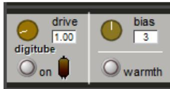
DiGiTube emulates the non-linearities of a valve amplifier: At low levels the valve is almost linear and at high levels the valve starts to compress and exhibits ‘soft clipping’.
